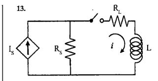
In the above circuit, the switch is closed at t = 0. The rate of change of current  $\frac{di}{dt}$  (0<sup>+</sup>) is given by
