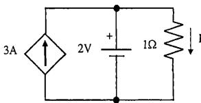
The current 'I' flowing through the  $1\Omega$  resistance in the above circuit is
