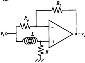
The transfer function  $[v_o(s)/v_i(s)]$  of the above circuit is
