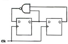
For the counter circuit shown in the Figure above, the Counter State  $(Q_1Q_0)$  will follow the sequence
