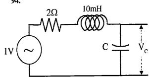
The series LCR circuit shown in the figure above resonates at  $\omega = 1$  k rad/sec. The voltage  $V_c$ across the capacitance at resonance is
