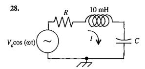
As the signal frequency ' $\omega$ ' in the above circuit is changed keeping the signal amplitude  $V_0$  constant, the current 'I' through the circuit exhibits a peak at angular frequency  $\omega=10^4$  rad/sec., with FWHM of 200 rad/sec. The value of the resistance 'I' is
