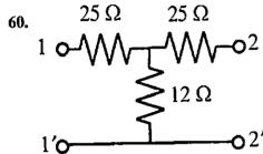
The characteristic impedance of the 2-port network shown in the figure above is
