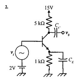
In the above amplifier circuit, the capacitors  $C_E$  and  $C_C$  have negligible reactance at the operating frequencies. The small signal gain  $(v_O/v_i)$  of the amplifier is
