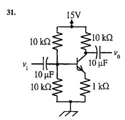
The transistor in the amplifier circuit above has  $h_{fe} = 100$ . The small signal mid-band voltage gain of the amplifier  $(v_o/v_i)$  is
